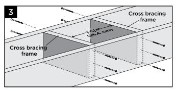
3. Install two 2" x 8" (51 mm x 203 mm) cross bracing frames in between joists at 7-1/4" (184 mm). Attach a total of twelve 3" (76 mm) pressure-treated compatible screws *(not provided)*.
