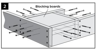
2. Install two 2" x 8" (51 mm x 203 mm) boards as blocking under post location. Securely attach blocking using a total of twenty-four 3" (76 mm) pressure-treated compatible screws (*not provided*).
