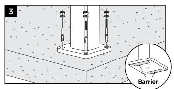
Insert (2) stainless steel barrier stripes under mounting bolt holes. Use appropriate shims if posts are not plumb. Attach posts using four TREX SUPPLIED 3/8" x 3-3/4" (10 mm x 95 mm) wedge anchors. Reference SKU part number ALPOSTHWCONC for required hardware (wedge anchors, washers, and nuts).
