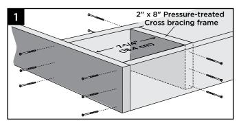
Install 2" x 8" (51 mm x 203 mm) cross bracing frame in between joists at 7-1/4" (184 mm). Attach a total of twelve 3" (76 mm) pressure-treated compatible screws (*not provided*).
