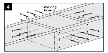
4. Install two 2" x 8" (51 mm x 203 mm) boards as blocking under post location. Securely attach blocking using a total of twenty-four 3" (76 mm) pressure- treated compatible screws (*not provided*).
