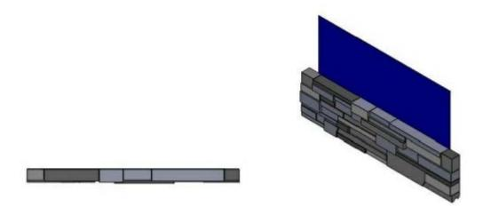
FIGURE 1—SILVERMINE STONE® VENEER PANEL AND ALUMINUM FLASHING
