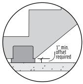
**Note:** A raised base plate will inhibit moisture in the concrete slab (or surrounding area) from absorbing into and eventually destroying the wooden stringer.
