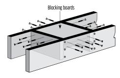
Using the post as a template, mark hole locations and drill through decking and blocking boards.
