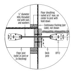
DTT2Z Installed as a Lateral Connector for a Deck-to-House Lateral Load Connection.
