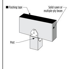
FIGURE 2B. Post-to-Beam Attachment
