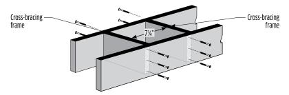
Install two 2x8-inch blocking boards under post location. A total of 24, 3-inch screws must be attached.
