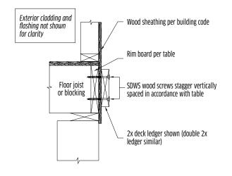
Ledger-to-Rim Board Assembly (Wood-framed lower floor acceptable, concrete wall shown for illustration purposes)
