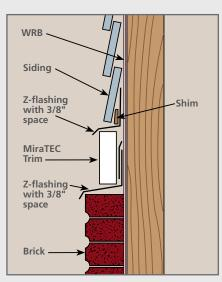
Install flashing in a manner that creates proper out-sloping.
