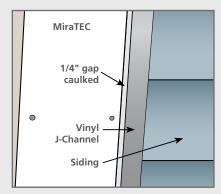
Vinyl J-Channel: Maintain a min 1/4" gap and fill with caulk where the MiraTEC butts against vinyl j-channel. This applies for both vertical and horizontal applications of trim and j-channel. Vinyl J-Channel is not a substitute for flashing.
