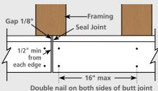
Double hall on both sides of butt joint
