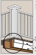
When facing the skirt boards on deck, properly flash the top edge to prevent water from getting behind the trim.
