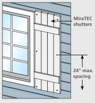
MiraTEC trim can be used to make decorative shutters. The shutter must be fastened to the home a minimum of 24" on center around the perimeter of the shutter as shown in the illustration. Working shutters are not covered by the MiraTEC limited warranty based on the inability of providing adequate fastening on the non-hinge side of the shutter.
