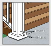
Properly flash and space at least 1/2" from any flatwork (such as porches, patios, decks, or driveways) or horizontal brick ledge. Prime and paint bottom edge before installing. Also all miter joints should be glued or caulked.
