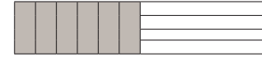
Main beams parallel to room's short dimension. Main beams parallel to room's long dimension.
