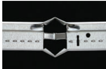
Main beam exposed to fire
