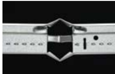
Main beam exposed to fire
