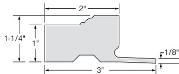
**BRICKMOULD WITH NAIL FIN**
