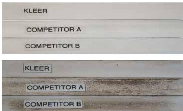
*Results from a dirt intrusion test show how much easier Kleer is cleaned compared to competitors.*
